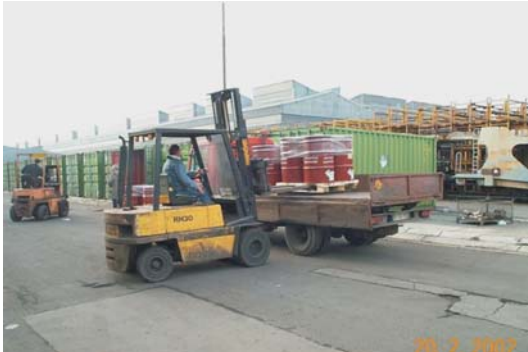
Loading of hazardous waste (HW) drums into containers and securing the loading, ready for transportation, February 2002
