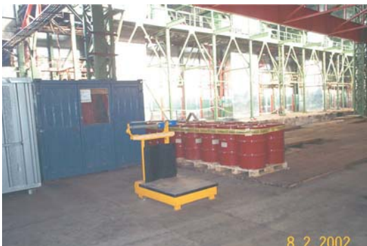
Sludge from paint hall pits packed in UN-approved Drums, February 2002
