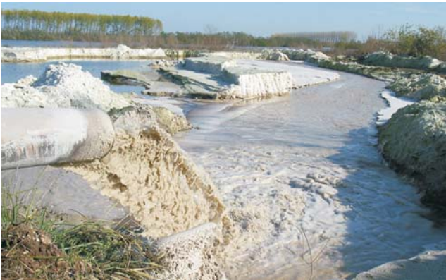
Wastewater discharge and storage of gypsum slurry next to Sava River, Zorka industrial complex, Sabac
