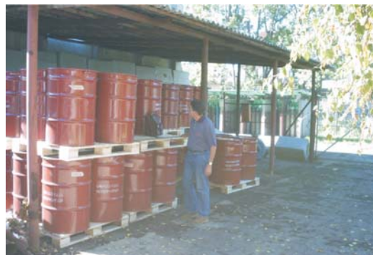
PCB-contaminated material packed in UN-approved drums for temporary storage, October 2002
