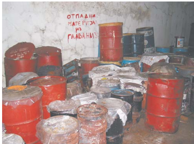
Storage of hazardous waste from galvanizing plant, Zastava
