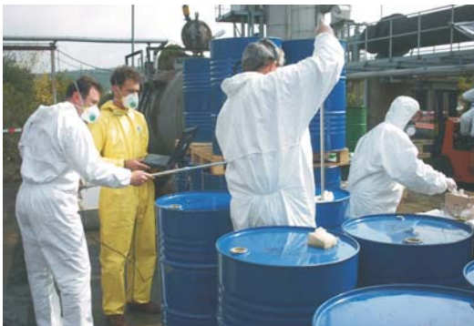
Sampling and packing of PCB- oil at Baric, September 2002
